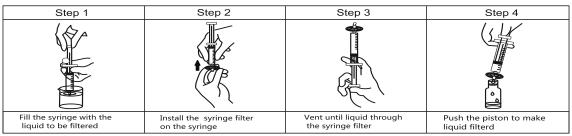
Fig. 1 ANOW \*syringe filter operation
